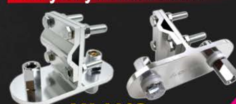
AM-1102 DUAL 3-WAY ALUMINUM ANTENNA MOUNT With One SM-1 Stud and One Down Stud For Ground, Mounts On Mast Up To 1 1/8" Diameter For 2 Mobile Antenna. One Side: SO-239 To 3/8-24T Mount Hole One Side: 3/8-24T Mount Hole
