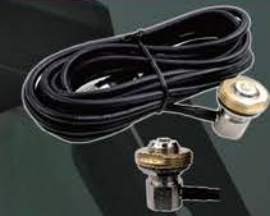
AM-207C-14 W/ 14FT. Cable AM-207C-17 W/ 17FT. Cable For 5/8" Mounting Hole NMO Right Angle Antenna Mount RG-58U Cable W/ Molded PL-259 Plug
