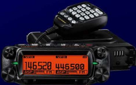
144/430MHz Dual Band 55W/50W FM Transceiver
