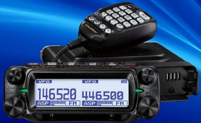
C4FM/FM 144/430MHz Dual Band 55W/50W Digital Transceiver
