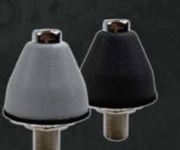
Antenna Trunk Hole Mount, SO-239 Connection, 3/8" x 24T Fitting.
