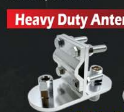
AM-1102 DUAL 3-WAY ALUMINUM ANTENNA MOUNT With One SM-1 Stud and One Down Stud For Ground, Mounts On Mast Up To 1 1/8" Diameter For 2 Mobile Antenna. One Side: SO-239 To 3/8-24T Mount Hole One Side: 3/8-24T Mount Hole
