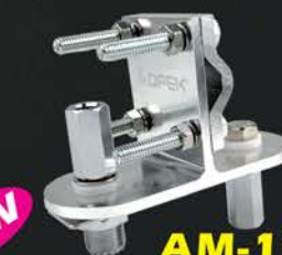
AM-1103 DUAL 3/8"-24, ALUMINUM DIPOLE MOUNT, W/ Connecting Plate Mounts On Mast Up To 1 1/4" Diameter For 2 Mini Dipole Antenna One Side: SO-239 To 3/8-24T Mount Hole One Side: 3/8-24T Mount Hole
