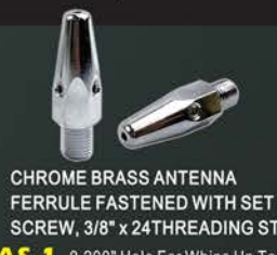
CHROME BRASS ANTENNA FERRULE FASTENED WITH SET SCREW, 3/8" x 24THREADING STUD. AS-1 0.200" Hole For Whips Up To 102". AS-2 0.100" Hole For Whips Up To 60". AS-3 0.125" Hole For Whips Up To 80".
