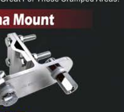
AM-1102 DUAL 3-WAY ALUMINUM ANTENNA MOUNT With One SM-1 Stud and One Down Stud For Ground, Mounts On Mast Up To 1 1/8" Diameter For 2 Mobile Antenna. One Side: SO-239 To 3/8-24T Mount Hole One Side: 3/8-24T Mount Hole
