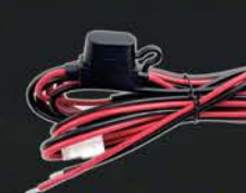
OP-KEN10HWP 2-Pin Kenwood NX Connector To Tinned End KENWOOD 10FT 14AWG 2-WIRE CB POWER CORD W/ INLINE FUSE BOX (15A Fuse) (15cm To The Fuse Box)
