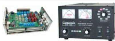
HF + 6, 1200 W Solid State Amplifier ALS-1306
