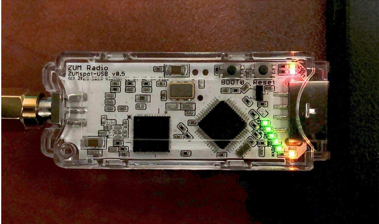
Insert the ZUMspot USB into any of the USB ports on your Windows machine. All of the LEDs will flash when first powered on and the PWR LED will remain on. Also, if you have the sound enabled on your computer, you should hear the USB device enumerate twice.
