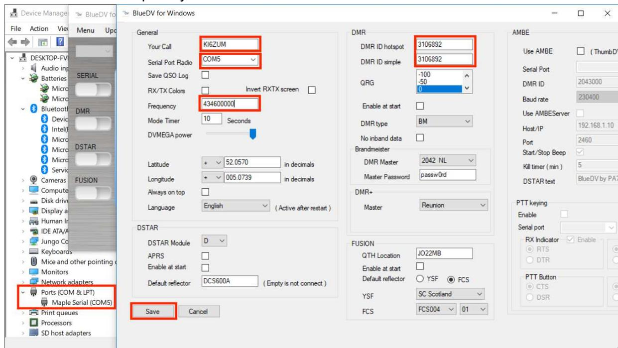
**NOTE:** If you reconnect the ZUMspot to another USB port, it may enumerate under a different COM port. So whenever you reconnect, double check your “Setup” with the COM port under Windows Device Manager.
