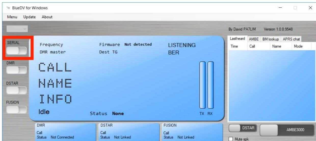
If the USB connection to the ZUMspot USB is functional, the software should display the “Firmware” version of the ZUMspot.
