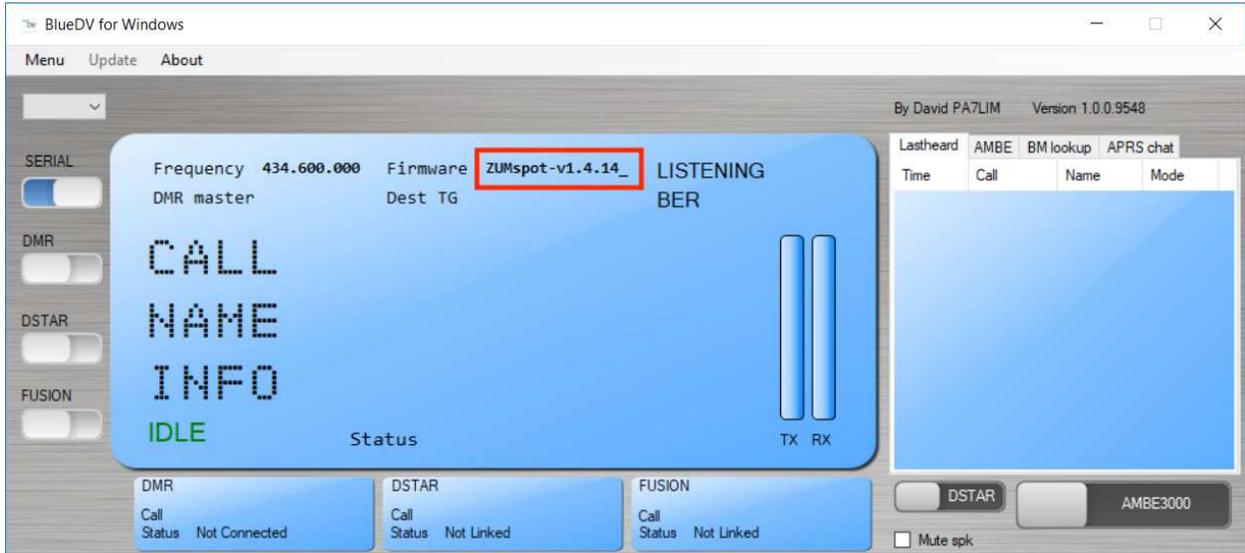
For DSTAR, turn on the DSTAR button, select the reflector (“REF”) you wish to connect to and then select “Link”
