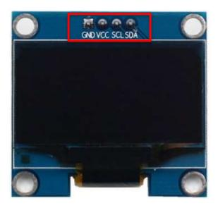
The ZUM AMBE3000 board has an OLED port with 4 pins (GND, 3V3, SCL and SDA). A 4 pin header should be soldered to the board. The 4 pins should be connected together:
