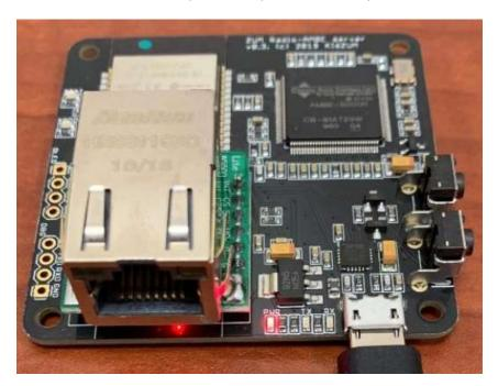
When using Wi-Fi or Ethernet mode, it is recommended to use a 5V USB power supply with at least 1A current rating. When using USB UART mode, it is recommended to use a powered USB hub. After applying power, the STAT and XCODE LEDs will flash up two times.
